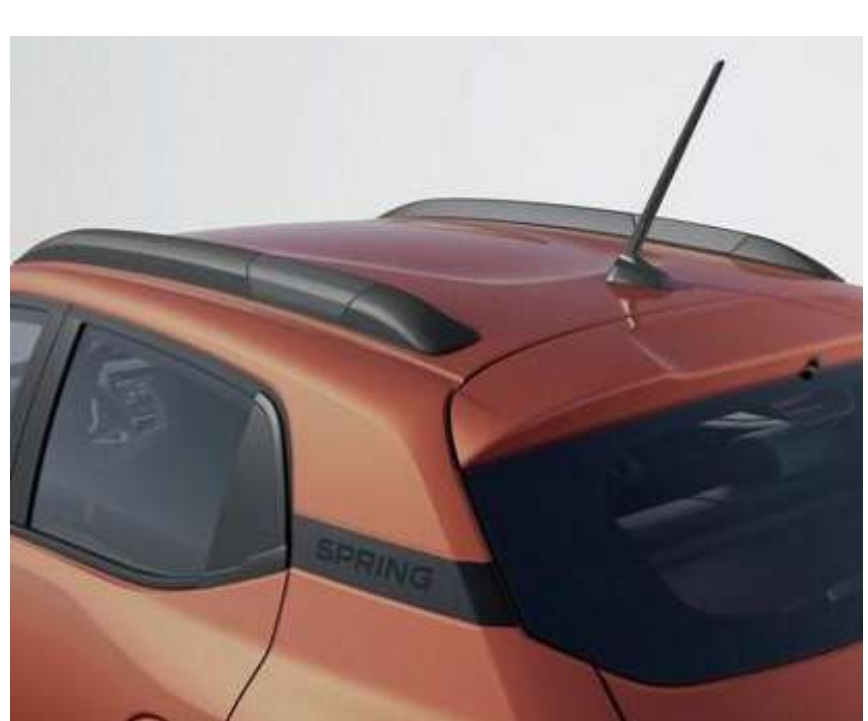
Decorative roof bars (Not load bearing)
