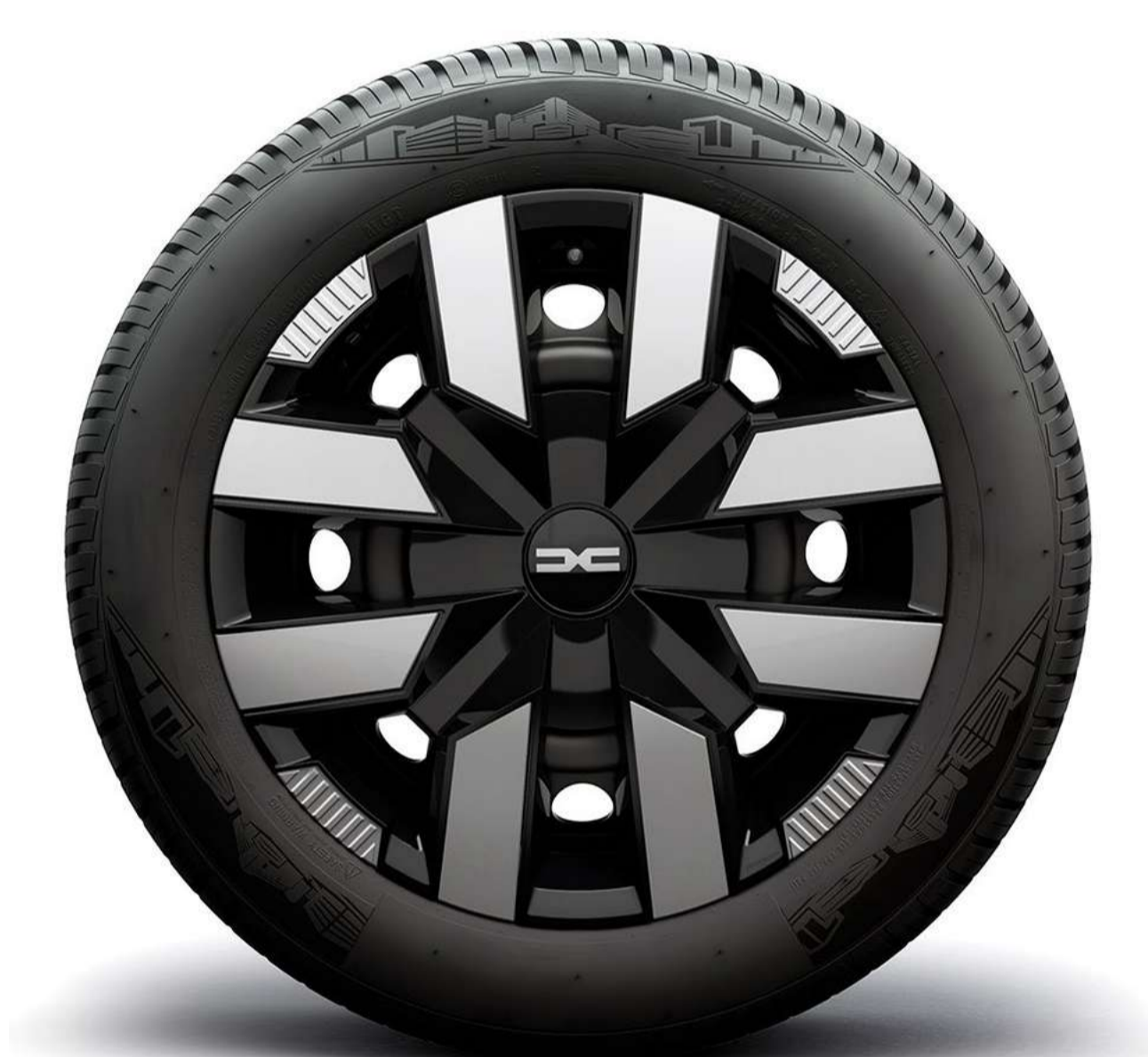
14" steel wheels with "Cians" styler (Standard on Electric 45 version) 15" steel wheels with "Resia" styler (Standard on Electric 65 version)
