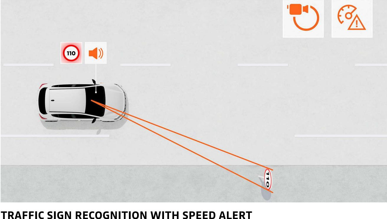
This system provides a reliable real-time indication of the maximum speed on the road and warns the driver if they exceed the speed limit with visual and audible alerts (which can be disabled).
